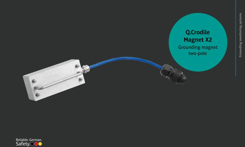
The Q.Crodile Magnet X2 was designed as a flat component. It can be used wherever safe grounding is required but there is not enough space for grounding clamps. The hand magnet is placed on the lid or on the side of the drum and held in place by magnetic force. The two built-in tips connect to the base of the drum with a little manual rubbing, creating a secure connection to good earth.
