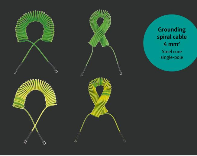
The single-pole, silicone-free steel core spiral cables from REMBE® offer superior mechanical strength. The steel core used can withstand continuous daily use and its cable sheath is extremely resistant to acids, alkalis, mineral oils, grease and other chemicals. In contrast to conventional copper cables, the stranded steel wire does not break due to continuous daily use.
